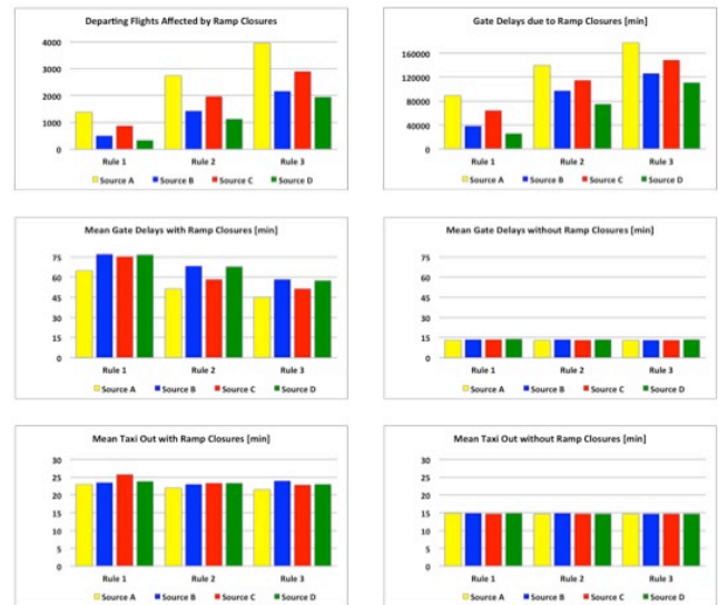
Fig. 4. Departure statistics from 1 January through 31 October 2013 for one major airport. Shown are the total number of flights affected by nominal ramp closures (upper left) and associated cumulative delays (upper right), mean gate pushback delays for flights affected by ramp closures (middle left) and those not affected by ramp closures (middle right), and mean taxi-out time for flights affected by ramp closures (bottom left) and those not affected by ramp closures (bottom right). Nominal ramp closures were computed based on four sources of lightning data (color coded) and three safety rules (grouped together).
