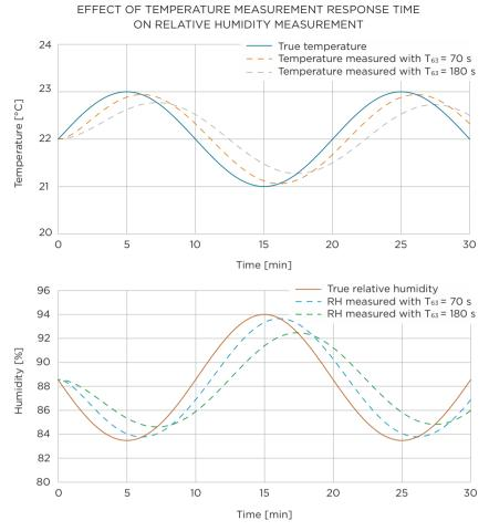
Figure 2. In the upper graph, the dashed lines represent the temperature readings of two instruments with different  $T_{63}$  response times in a slowly changing temperature. In the lower graph, the impact of the temperature measurement error on the relative humidity measurement is shown. The slow stabilization with respect to temperature causes an additional  $3 \dots 4$  %RH error in the relative humidity measurement.
