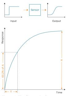
Figure 1. The first order linear time-invariant system
