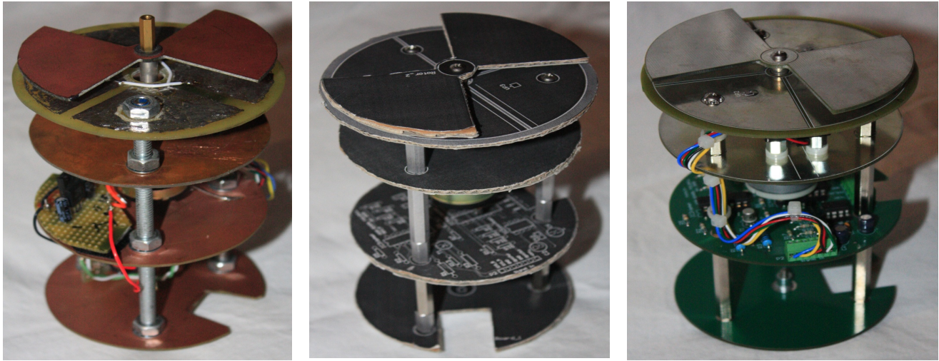
Figure 8. Comparison of hand-made alpha mill, cardboard mock-up, and "professionally" designed beta mill
