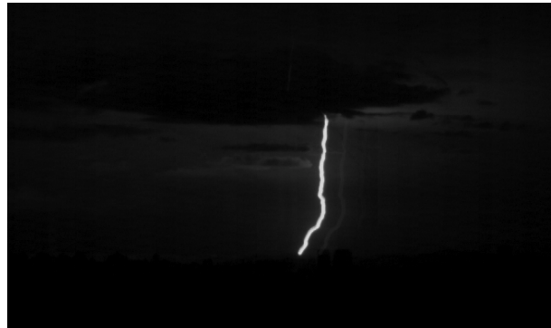
Figure 6. One frame from a flash with a very long continuing current of more than 600 ms, recorded by the RAMMER sensor.
