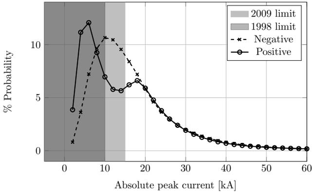
Figure 2: Discrete probability density functions computed from the cloud-to-ground data set.
