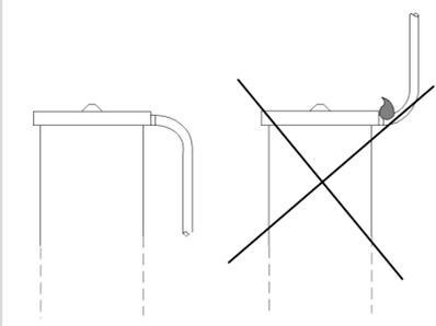
PTB210 has IP65 housing. You can mount it outdoors without any additional protection. Make sure that rainwater cannot block the open pressure fitting. Vaisala recommends connecting a piece of a tube with inner diameter of 4 mm or more to the fitting.
