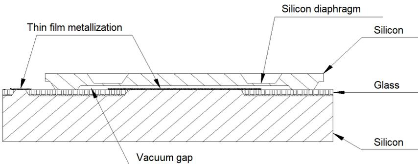
Figure 2 BAROCAP pressure sensor
