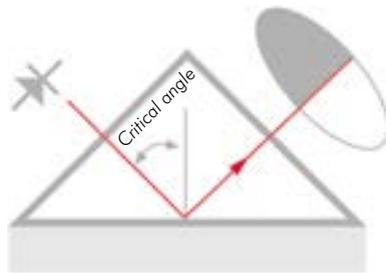
A digital CCD-camera detects the optical image and the shadow line. The camera transforms the optical image point-by-point to an electrical signal. The exact shadow line position is located and converted to a reading in refractive index.
