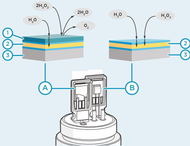
**A** HUMICAP sensor with a catalytic layer (under the probe filter). This sensor only senses water vapor.
