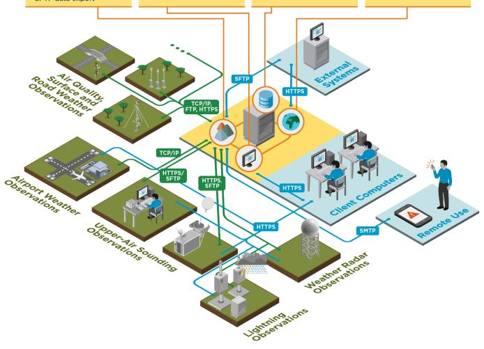
NM10 is a stand-alone system installed in customer premises on Windows or Linux operating systems. The system is configured individually for each customer use. The figure shows the available main components and interfaces of the system.
