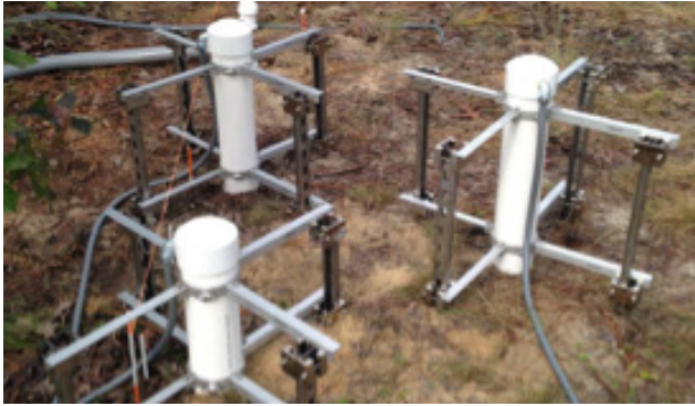
GMP343 sensors are located inside access tubes within a soil plot (Source: NEON Doc. #: NEON.DOC.003633 NEON Preventive Maintenance Procedure: Soil CO 2 Concentration)
