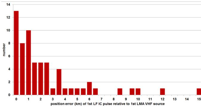
**Fig. 4. Distribution of position errors between the first LMA sources and first pulses in pulse trains occurring at preliminary breakdown**
