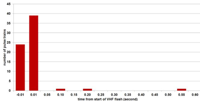
Fig. 3. Distribution of the time difference between the start of LMA flashes and the first pulse in a train with multiple geolocations.
