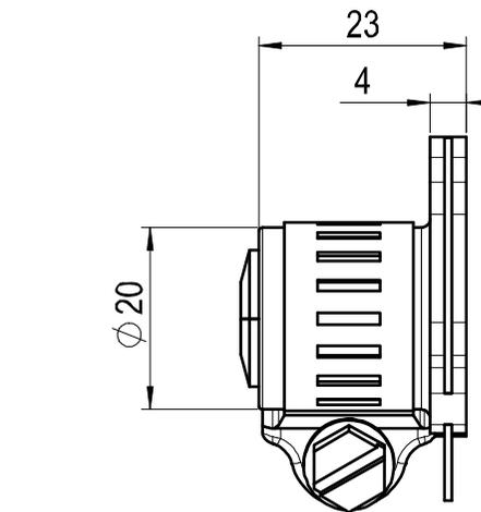
Figure 5 Mounting Flange Dimensions
