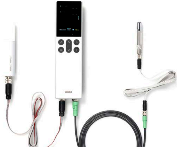
Indigo80 with GMP251 carbon dioxide probe and HMP110 humidity and temperature probe. The HMP110 probe offers measurement accuracy from \pm 1.0 °C and \pm 1.5 %RH (0... 90 %RH) with higher accuracies available. The GMP251 CO 2 probe provides accuracy from \pm 0.1 %CO 2 depending on operating conditions.
