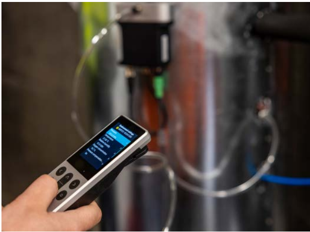
Indigo80 handheld device with GMP80P pump & tubing
