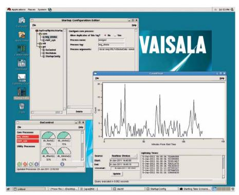
The FALLS® Server is a processing module in the Vaisala Thunderstorm Information System that specializes in archiving cloud and cloud-to-ground lightning data for forensic applications, and connecting with the FALLS® client application to display decision support information.
