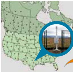
*U.S. NLDN consists of the latest advanced ground-based lightning sensor technology from Vaisala.*
