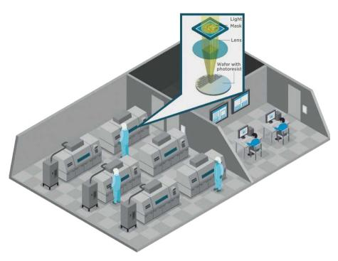
Precision air conditioning and wafer stepper process capacity can be significantly enhanced with accurate and stable measurement of air pressure, temperature, and humidity. Wafer manufacture requires a highly controlled environment and precise data on the manufacturing environment. These essential elements enable **both high accuracy** and **high speed** of the circuit pattern exposure on the wafer surface.
