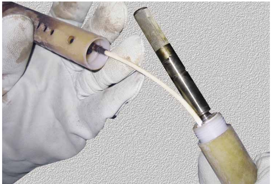
HMT330WPA cover protects humidity probe from any water splashes or dirt.
