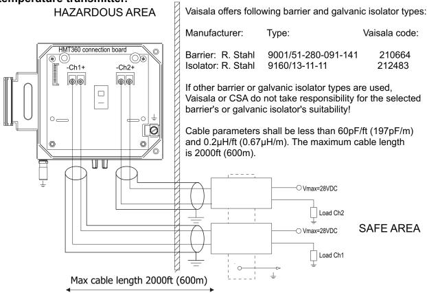
HMT360-series transmitters are approved for use in Division 1 and 2, Class I, Groups A, B, C, and D. Division 1, and 2, Class II, Group G and coal dust. Division 1, and 2, Class III.
