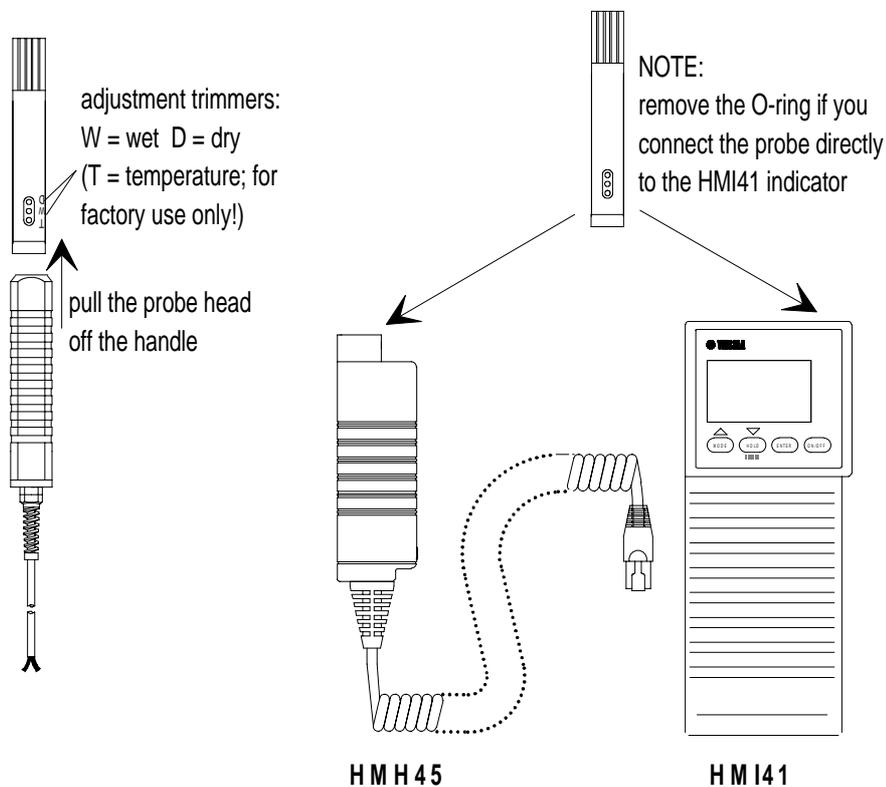
**Figure 2 Adjustment trimmers and probe head connection/disconnection**
