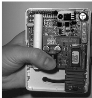
Figure 2: Installing the GML20T module
