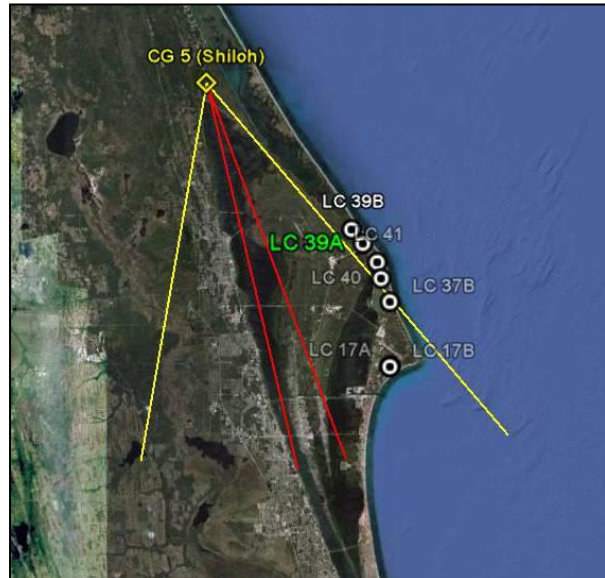
(a) Sectors in which the detection rate of the Shilo sensor is degraded.
