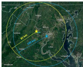
Fig. 3. Map of the KLWX radar range ring (yellow) and the Washington, D.C. LMA range ring (blue) overlays. The stars denote the range ring centers.
