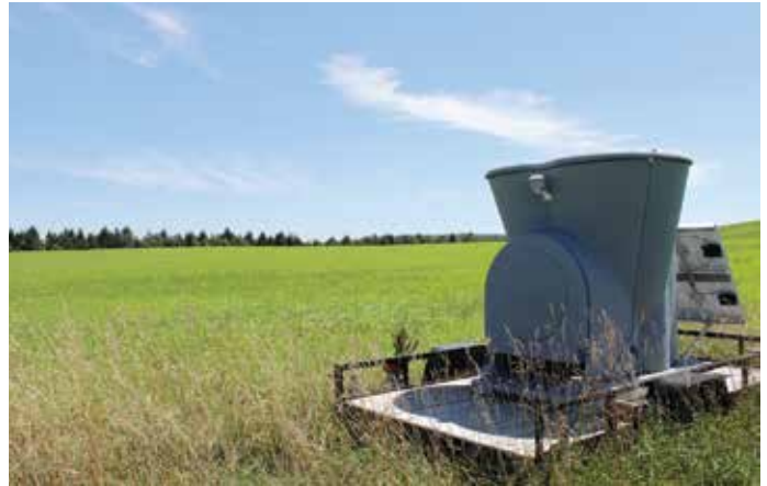
EverPower uses Triton Wind Profiler as part of its wind resource assessment program to dramatically reduce uncertainty in wind resource and project energy estimates.
