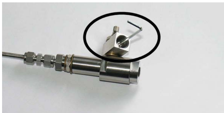
Figure 15 Removing the Leak Screw
