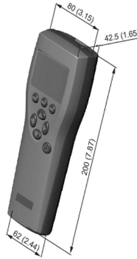
MI70 dimensions in millimeters (inches)
