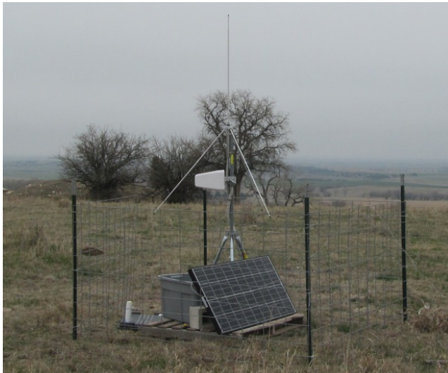
Fig. 4. Portable Lightning Mapping Array (LMA) Station.
