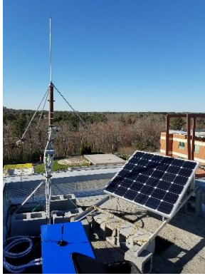
Fig. 2. NGLMA system setup, including the antenna, GPS, PC104-based processing system (in blue box), cell phone antenna, and solar panel.
