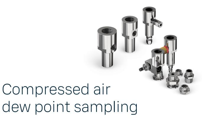
Sampling is needed when direct measurement of the air is undesirable or is simply not feasible. This may be due to a high process temperature, the need to protect the sensor from water spikes, the added convenience of installing and removing the instrument from a pressurized process without shutting down the line or wanting to make the measurement in a more convenient location.
