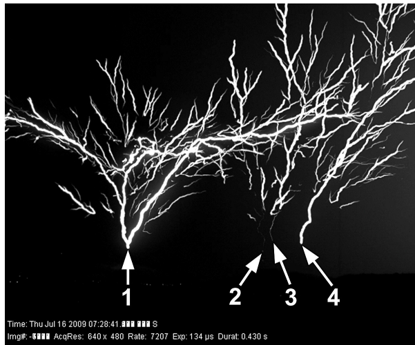
Figure 9. Time-integrated video segment from a high-speed camera (7.207 ips, 134 exposure) showing the prolific development of bright RLs on the weakly luminous branches of four UPLs. Many of the RLs faded prior to connecting to the main stem.
