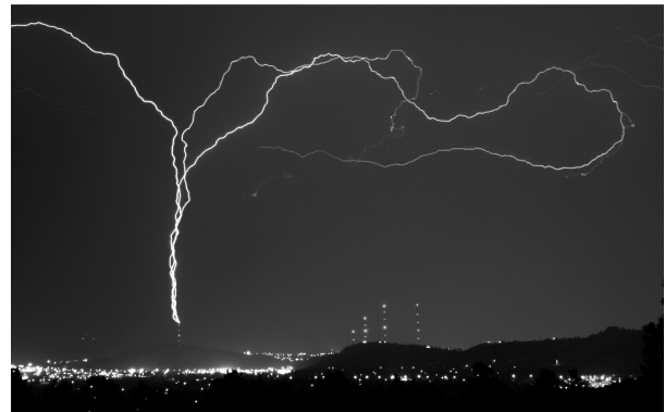
Figure 10. A composite image of three upward flashes photographed with a digital still camera (20 sec exposure). All three non-branched UPLs initiated from Tower 1 and transitioned to horizontal propagation below cloud base.
