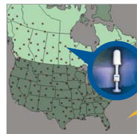
CLDN consists of more than 80 remote, ground-based Vaisala lightning sensors
