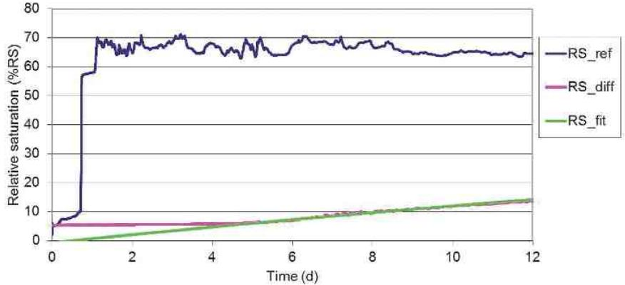
Figure 3. Relative saturation in the measurement line ( $RS_{ref}$ ) and in the side tube ( $RS_{diff}$ ), and best fit of Equation 1 to  $RS_{diff}$  (named  $RS_{fit}$ ). Distance from sensor head to oil flow is 17.3 cm.
