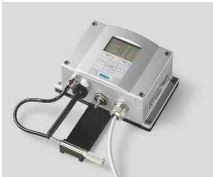
PTU301 short cable probe with optional WLAN
