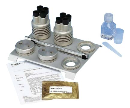
Vaisala Humidity Calibrator HMK15 - an example of a saturated salt bath device.
