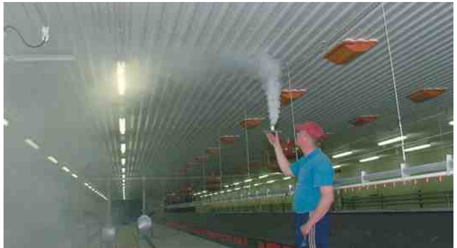
Smoke is used to visualize the air circulation inside an animal shelter in order to optimize the design of the ventilation system.
