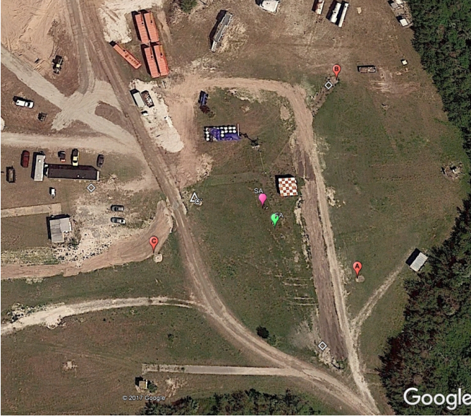
Fig. 1: A satellite image map showing the 2017 VHF antennas (red), fast antenna (green) and slow antenna (magenta) locations. The 2016 VHF antenna locations are marked with hollow white diamonds while a temporary VHF antenna C location used only on February 15, 2017 is indicated by a hollow triangle. The INTF PC data acquisition system was located within the building with the checkerboard pattern top.
