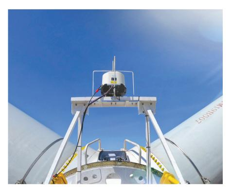
WindCube® Nacelle makes Lidar-Assisted Control (LAC) a reality, reducing Levelized Cost of Energy (LCOE) and creating numerous other benefits for wind energy.
