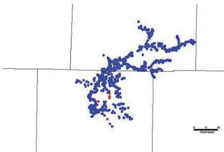
Cloud lightning flash detected in the Dallas-Fort Worth area of Texas, USA. The blue dots show VHF cloud lightning mapping and the red dots show VLF/LF cloud lightning detection. The total length of this cloud flash as shown by VHF cloud lightning mapping is 50km
