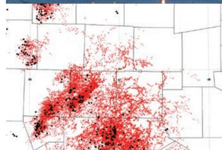
Map of VHF total lightning mapping in red and VLF/LF cloud pulses in black in north Texas for a 15-minute period. Note the large area of anvil lightning reaching northward from the center of the storm on the south side of the map
