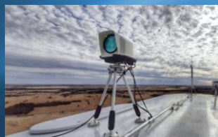
Fig.5 The photo of NML, installed on the turbine nacelle
