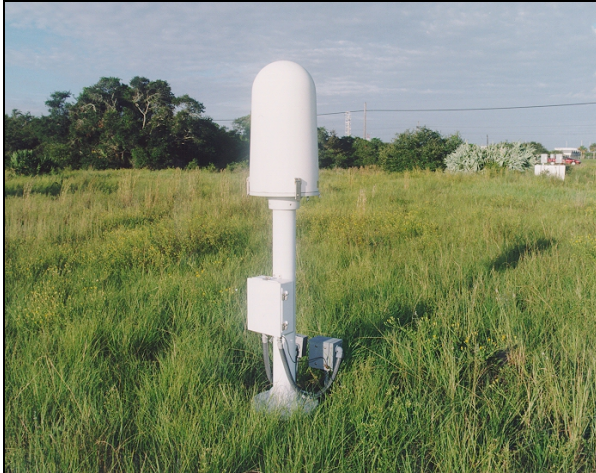
Figure 4. Picture of the sensor used in both the previous CGLSS-I and current CGLSS-II.
