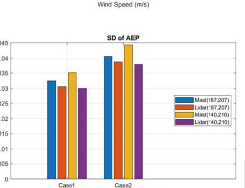
The difference of standard uncertainty in AEP is analyzed using two Weibull distributions, simulating different wind conditions at the test site. The left graphs show the standard deviation in AEP of the power curve measurements.
