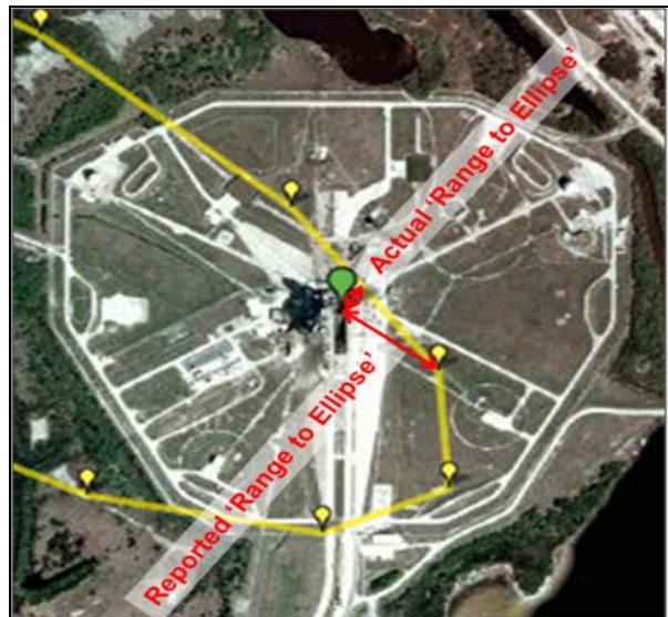
Figure 9. The previous method of estimating the distance from the facility to the closest point on the error ellipse was done using the distance to the closest of the 13 evenly spaced points used to approximate the ellipse. This method would grossly over-estimate the distance when the facility was close to the ellipse and about equidistant from the two closest 13 points. This method was replaced by a far superior method as discussed in the text and shown in Figure-10.
