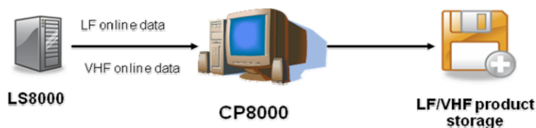
Fig 2. On-line storage of the data detected by the LS8000 sensors.
