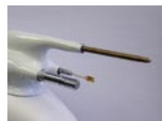
Figure 2: Meteorological probes mounted in the noseboom of the T200.
