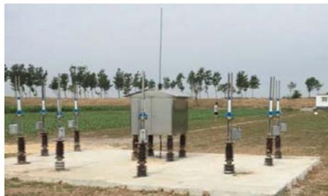
Fig. 2. Installation of rocket-triggering lightning experiment in Zhanhua, Shandong (SHATLE).
