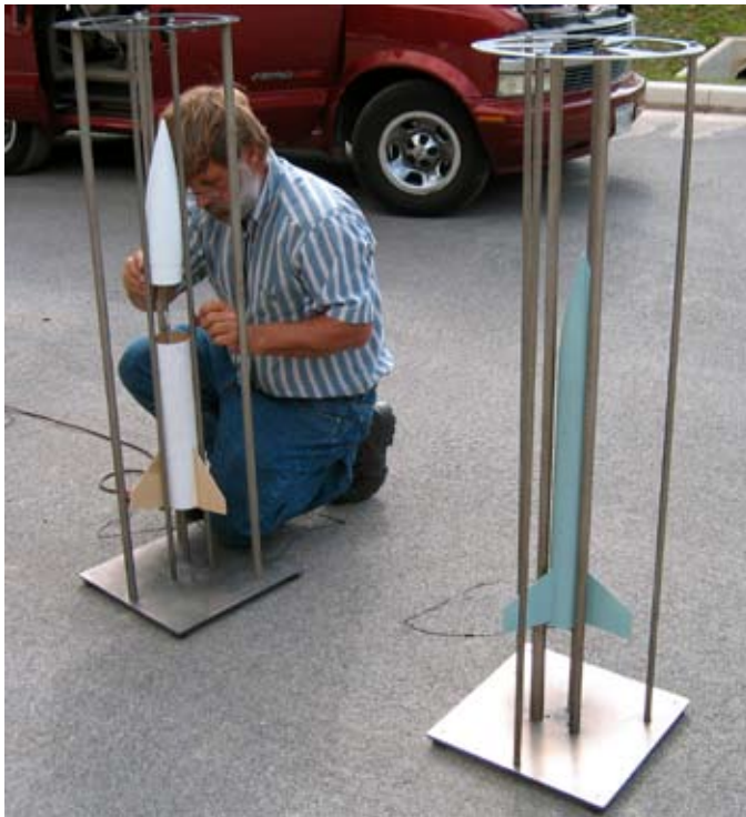
Figure 2. JHU/APL rocket scientist, Charles Etheridge prepares 3-inch back-fit rocketsonde for launch. A 2.5-inch back-fit rocketsonde is ready on the right.
