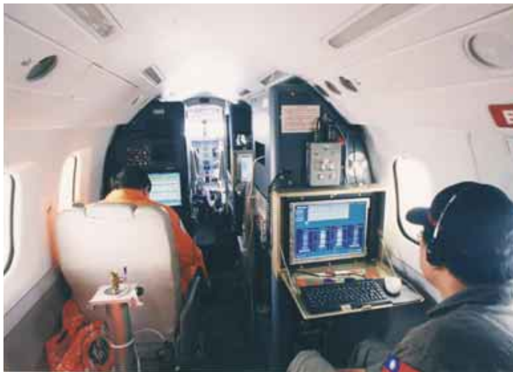
The interior of the Astra, with the Vaisala AVAPS Dropsonde Receiving System located in the center right, and the dropsonde launcher to the lower left.
