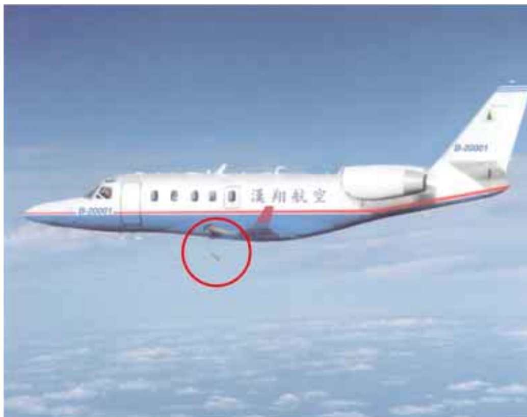
The Astra SPX jet releasing a dropsonde (circled) during a test flight in March, 2003.
