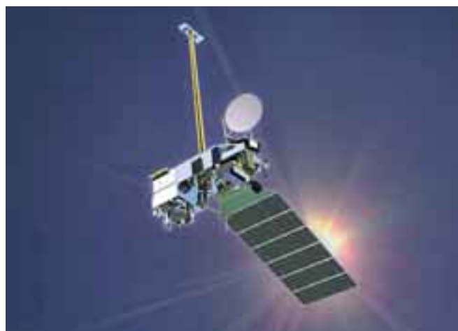
Meteorological exploration by satellite can be either passive (measures on natural radiation in frequency bands that depend on physical laws) or active for physical measures (altimeters, cloud profiling and precipitation detection).
