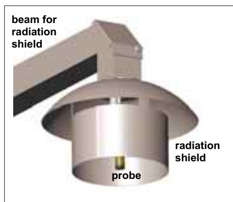
The dewpoint probe in the specially designed radiation shield with open structure.
