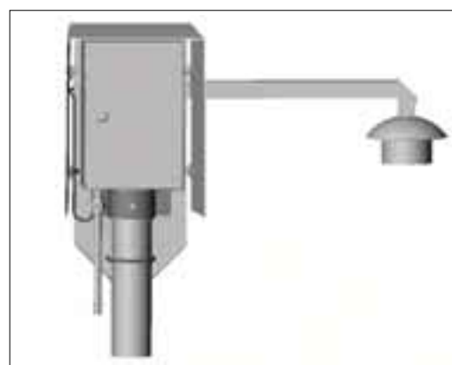
The dewpoint measurement in the ASOS network at NWS incorporates an installation kit for the sensor head together with an enclosure for the dewpoint transmitter and optical modem. The warmed probe of the transmitter is installed in a radiation shield with open structure.
