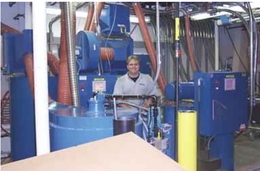
At Tessy Plastics, Todd Eaton uses Vaisala DM70 Hand-Held Dewpoint Meters to monitor the plastic dryers.
