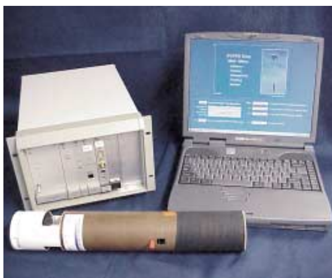
The AVAPS Lite is a compact system for airborne atmospheric data acquisition.
